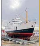
Cover photo: MV FRANCES BARKLEY, the first vessel lifted on Point Hope Maritime's new marine railway and vessel transfer system.
