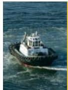
The tug **Tiger Sun** shows the high manoeuvrability gained from its azimuth thrusters – First Narrows, Vancouver.
